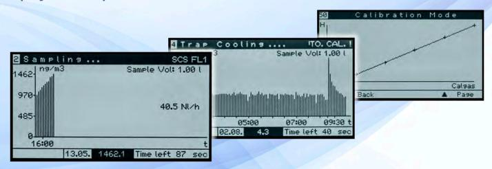
The results of the measurements are displayed on a graphic LCD as a graph and numerically. It is possible to view past readings with a paging function. Calibrations are stored in a non-volatile memory.
