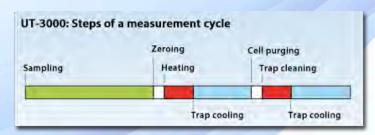
The use of air as a carrier gas is also advantageous during thermal Hg desorption as substances that could contaminate the system are oxidised and flushed out. This prevents any passivation of the gold surface.
